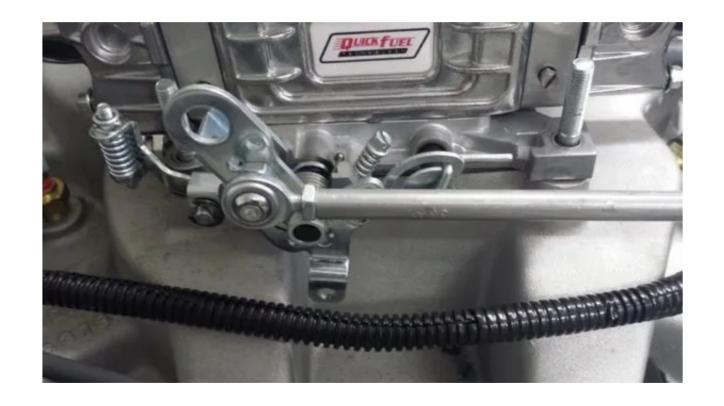
ATTACH THE ROD END ON THE THROTTLE LINKAGE OF YOUR CARB. WITH THE THROTTLE ROD SQUARE TO THE FIREWALL, MARK THE FIREWALL WITH A SHARPIE THE POSITION OF THE ALUMINUM LEVER.
