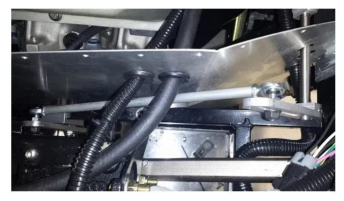
Align your gas pedal lever to where the throttle lever will be.
