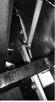
ALIGN YOUR GAS PEDAL LEVER TO WHERE THE THROTTLE LEVER WILL BE. THIS GOES OUTBOARD OF THE FIREWALL ROD END. MARK THAT POINT FOR THAT ROD END AND INSTALL ROD END TO FIREWALL.
