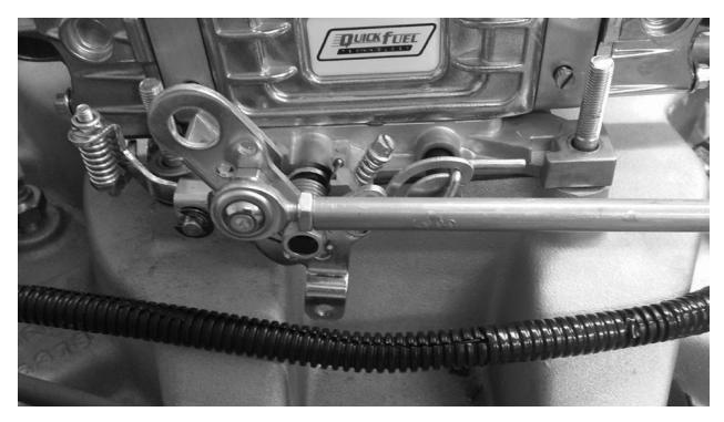
ATTACH THE ROD END ON THE THROTTLE LINKAGE OF YOUR CARB. WITH THE THROTTLE ROD SQUARE TO THE FIREWALL, MARK THE FIREWALL WITH A SHARPIE THE POSITION OF THE ALUMINUM LEVER.
